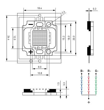
Note: all dimensions in mm tolerance is  $\pm 0.1$ mm unless otherwise noted.
