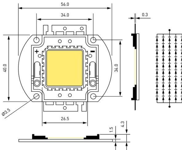
Note: all dimensions in mm tolerance is ±0.1mm unless otherwise noted.
