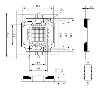
Note: all dimensions in mm tolerance is ±0.1mm unless otherwise noted
