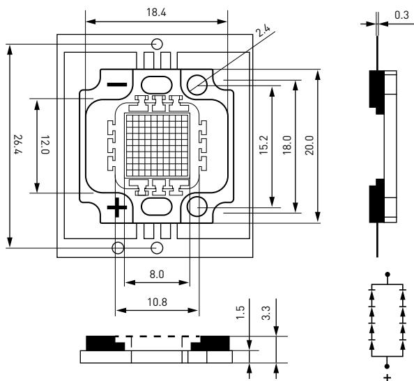
Note: all dimensions in mm tolerance is  $\pm 0.1$ mm unless otherwise noted.
