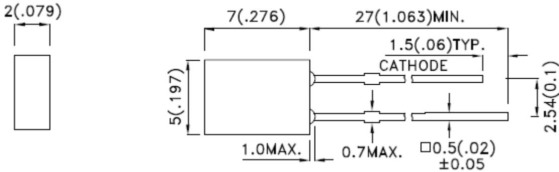
**Notes:** Other dimensions are in millimeters, tolerance is 0.25mm except being specified.
