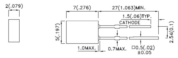
**Notes:** Other dimensions are in millimeters, tolerance is 0.25mm except being specified.
