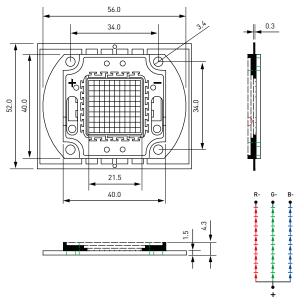
Note: all dimensions in mm tolerance is  $\pm 0.1$ mm unless otherwise noted.
